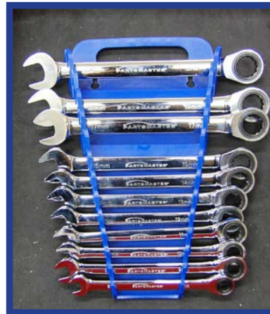
Allows visual observation of missing wrenches
