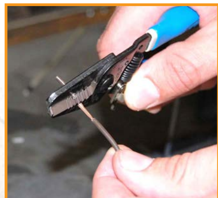
Strips stranded and solid copper and aluminum wire
