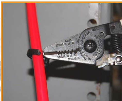
Cuts cable tie without damaging outer shield
