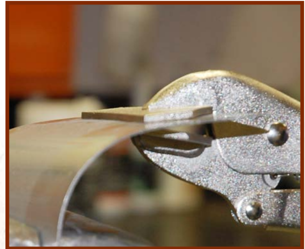
Allows bending and forming of sheet metal without a brake
