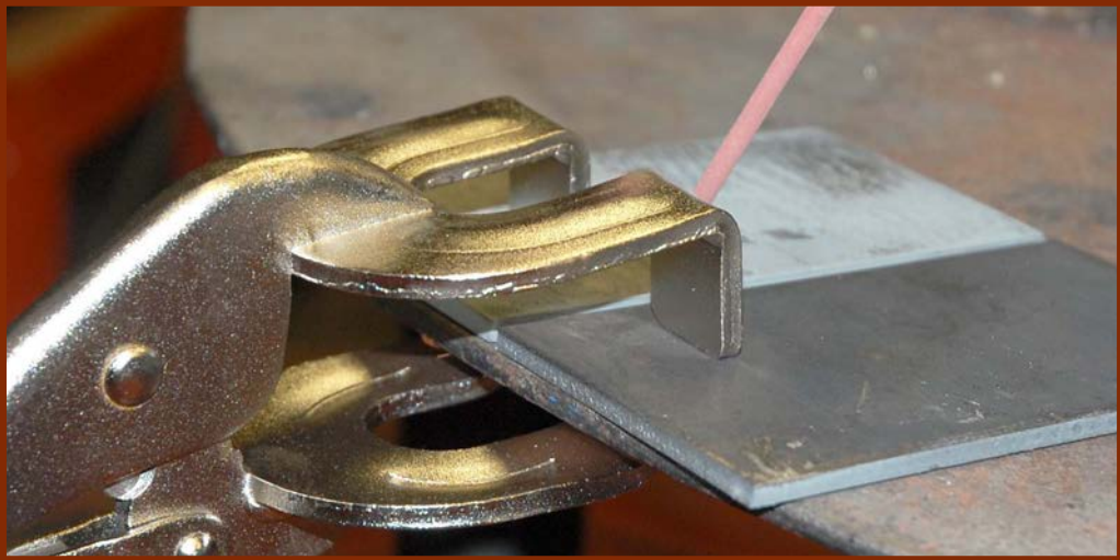
U-shaped jaw securely holds round, angled and flat material and allows access and visibility to the work area
