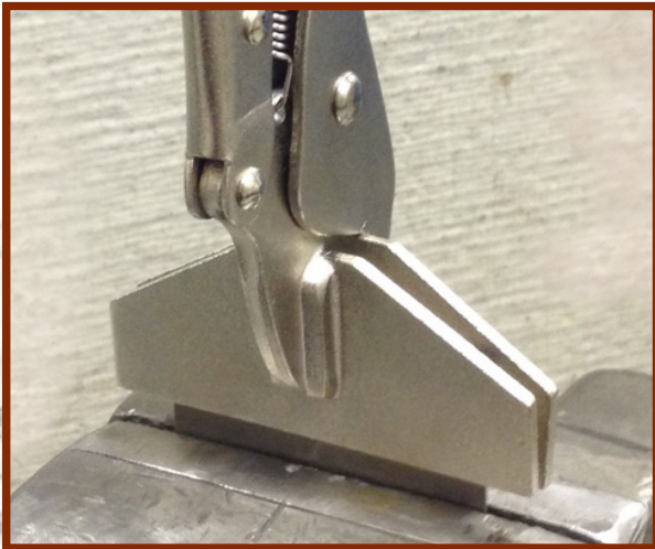
Allows bending and forming of sheet metal without a brake
