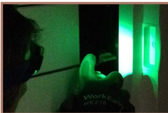
The green LED feature allows night crews to work outside and does not attract flying insects as easily as the white LED lights
