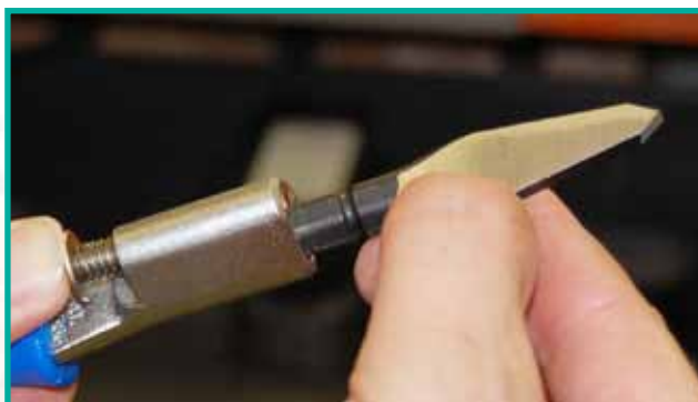
Lock and load feature on handle securely holds punches and chisels in place and allows fast, efficient style change outs
