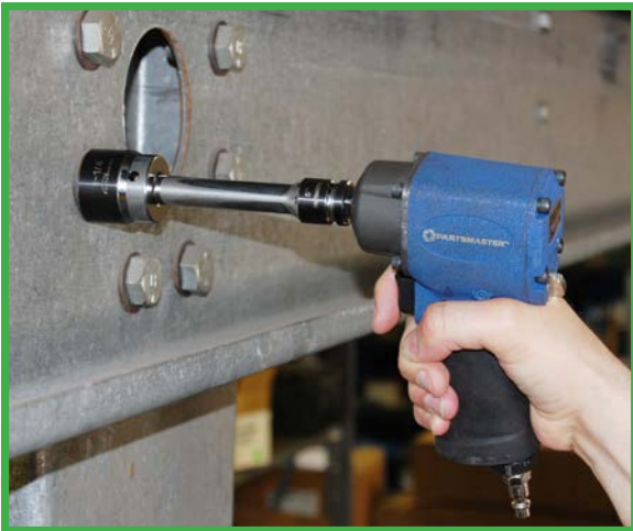
Can be used with standard drive tool, 18-volt ratchets, and pneumatic ratchets and impact wrenches
