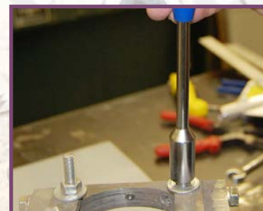
Deep well feature provides access to nuts attached to long threaded fasteners
