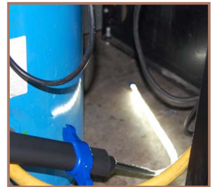
LEDs are positioned on both sides of the light wand, providing 360° illumination
