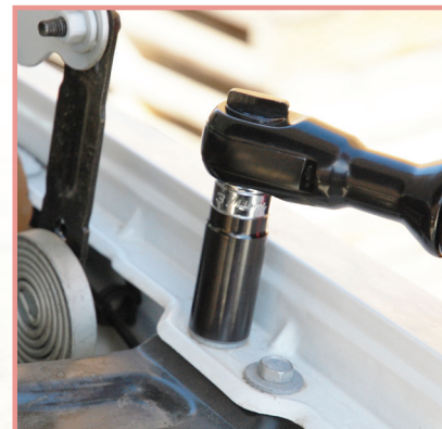
Air ratchets offer greater access to hard to reach areas than impact wrenches
